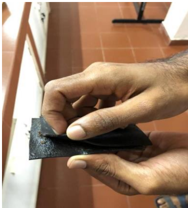
Fig. 8: Rubber pieces bonded together using adhesive
