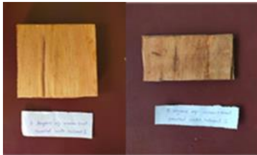
(a) 6 layer (b) 3 layer Fig. 7: Samples of veneer sheets bonded together
